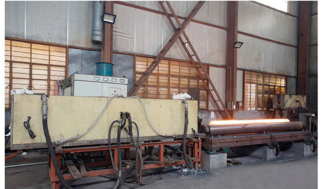
国际先进的大型合金离心浇铸设备 International advanced large bimetallic centrifugal casting equipment
